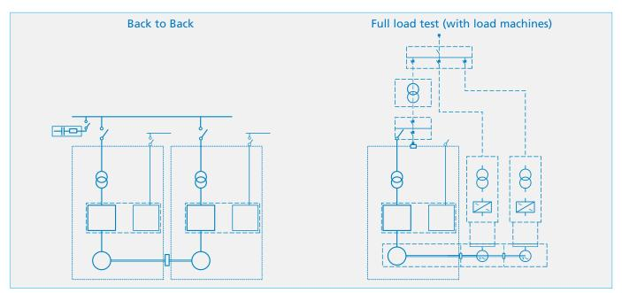
A thorough testing session shall be preferably held on the complete variable speed drive systems line-up before delivery at site in order to:
