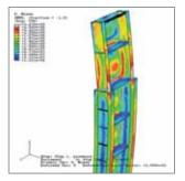
The confinement design can be verified against the blast pressure pulse using real-time dynamic analysis to check the maximum stresses and strains.
