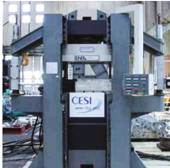
Machine designed and realised by ENEA for HDRB tests.
