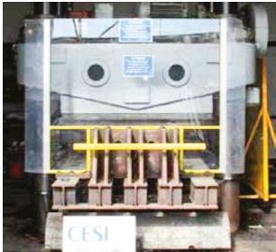
The machine can be assembled also for biaxial loads.
