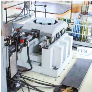
Specifically designed for HV bushings (seismic or short circuit stresses).
