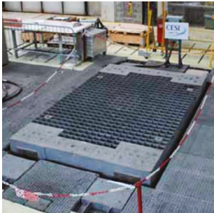
The machine can be assembled also for biaxial loads.
