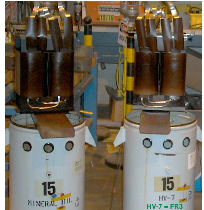
Transformers from cell A (167°C) after 5x nominal life
