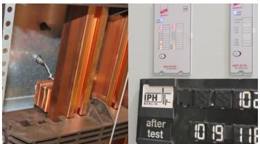
Ignition point and status indication of arc fault detection test
