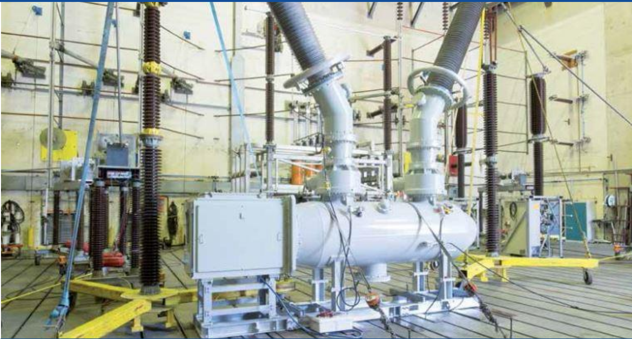
Testing of an SF6 alternative high-voltage circuit breaker at KEMA Labs
