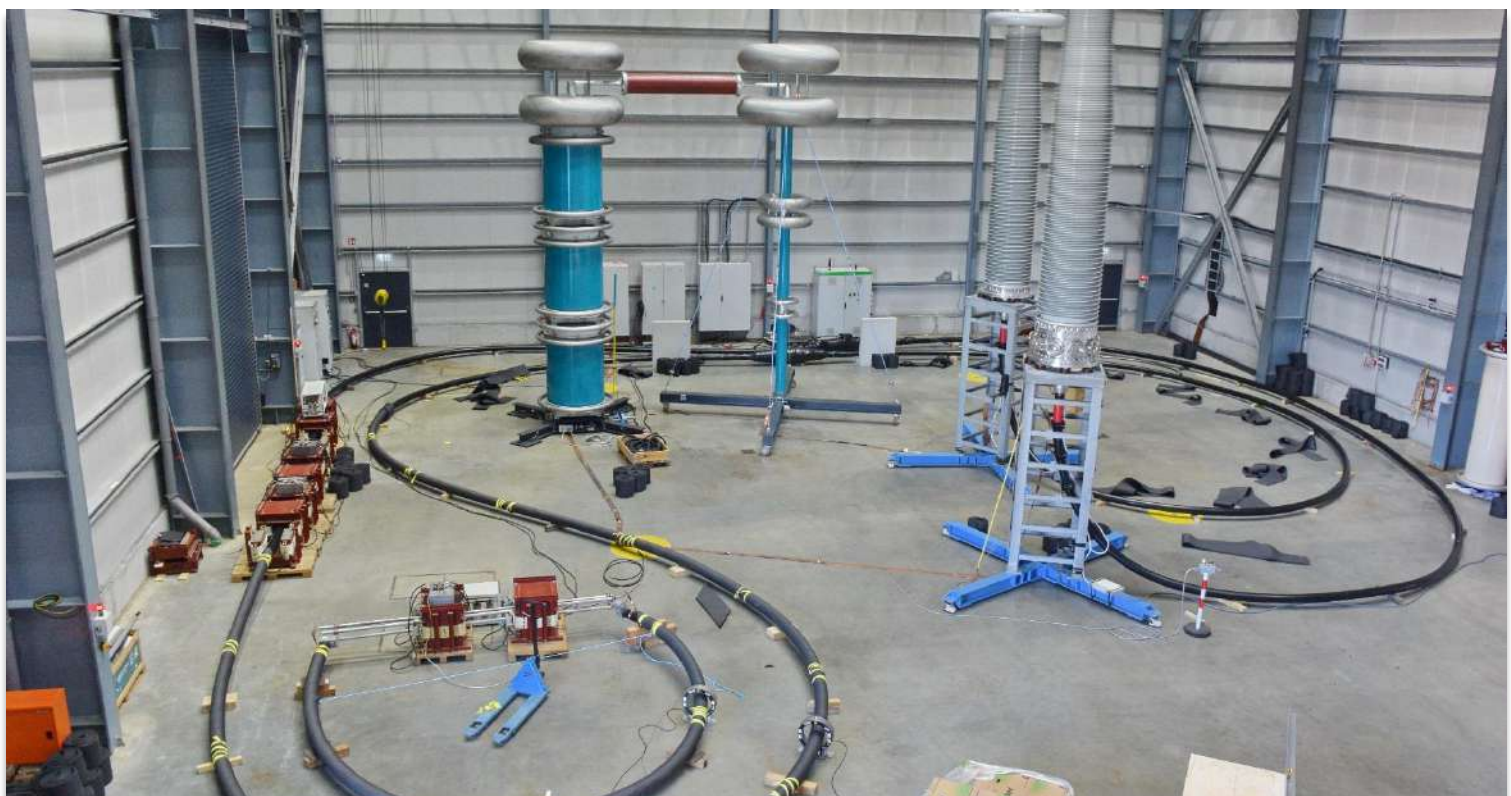
Dielectric testing of a 525-kV HVDC cable in a high-voltage laboratory of KEMA Labs, Mannheim Germany
