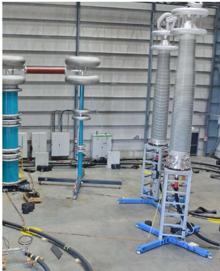
Dielectric testing of a 525-kV HVDC cable in high-voltage laboratory of KEMA Labs, Germany
