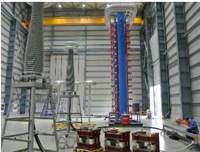
XLPE extruded cable with the Polarity Reversal tests performed up to 525 kV at KEMA Labs in Mannheim
