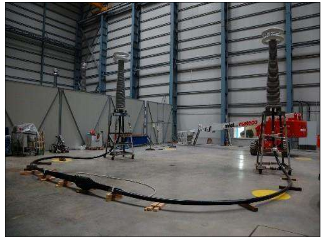
XLPE extruded cable with the Polarity Reversal tests performed up to 525 kV at KEMA Labs in Mannheim
