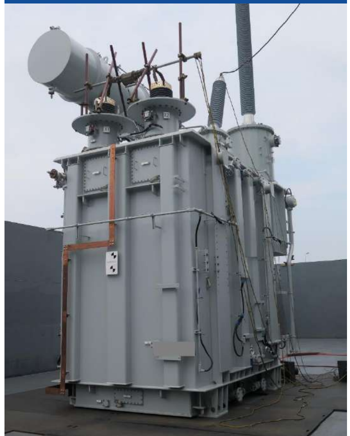
Transformer filled with natural ester under test, on the boat
