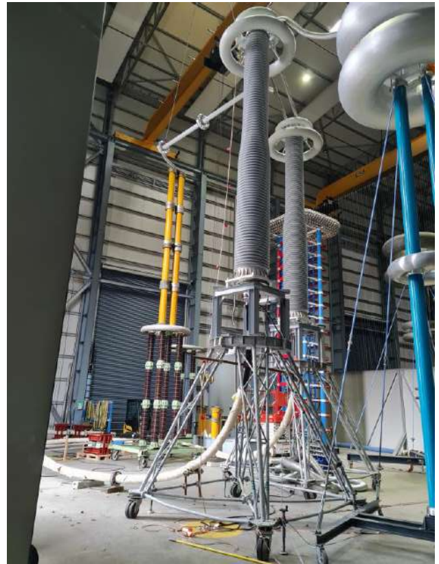
Reduced view of the test bay containing the set-up for TOV tests during the assembly phase
